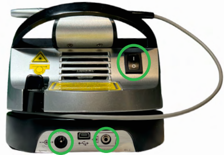
Figure 6.1: Power Switch, DC Power Input, Remote Interlock
